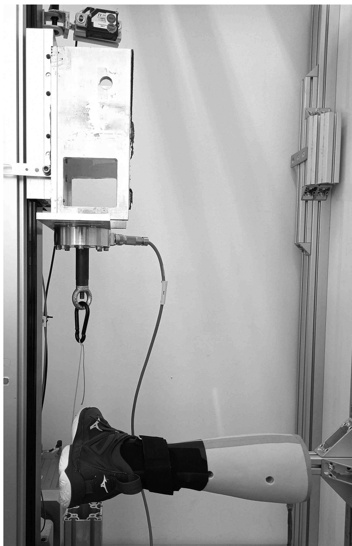
Figure 1. Mechanical tests performed with the artificial ankle (representing the right lower leg and foot) on the different brace conditions. Inversion is induced by pulling the rope connected to the lateral aspect of the foot upward. All braces were tested with the same shoe as during the biomechanical testing. Results represent the mean of 3 trials per condition.
